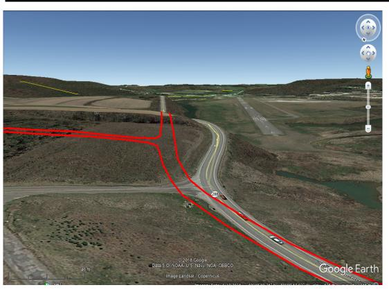
In order to reduce costs, the Airport Authority is performing excavation operations for the new location of SR 1010 without affecting the highways. The final portion of excavation will require SR 0288 and SR 1010 to be closed.
