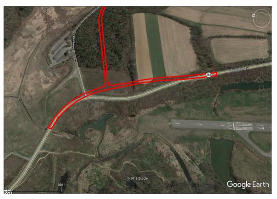
Realignment of 1,740-feet of SR 0288 will eliminate a reverse curve posted with an advisory speed limit and improve stopping sight distance to meet the minimum requirements. The highway will be lowered by as much as 50-feet.
